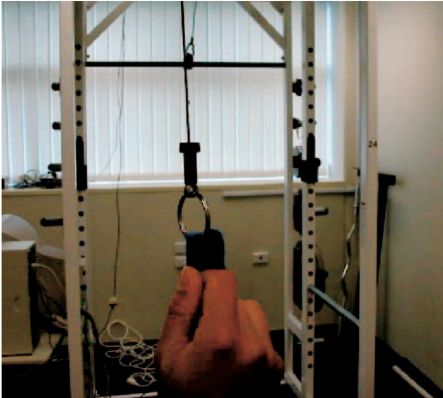
**Figure 2.** The cable end of the position transducer can be attached to the barbell.
