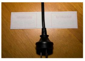
Wrap the label around the cable and tape in position
